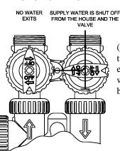
(Can be used as water turn off during extended periods when the home is not being occupied.)
