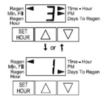
If the system has called for a regeneration cycle that day, regeneration will occur at the preset time for regeneration, an arrow on the display will appear pointing to "Regen".
