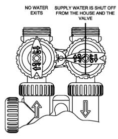
(Can be used as soft water turn-off during extended periods when the home is not being occupied.)
