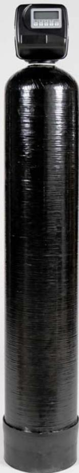
*The Iron Scrubber stores a bubble of air, within the media tank. As your water passes thru the air, the iron or sulfur is converted to a particle which is then trapped by the catalytic filter media in the tank while the air bubble is gradually consumed by the passing water. During regeneration, the unit first backwashes any oxidized iron particles it has trapped to drain. The system then replenishes the air bubble by drawing in oxygen from the atmosphere.*
