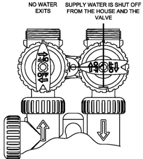
(Can be used as soft water turn-off during extended periods when the home is not being occupied.)
