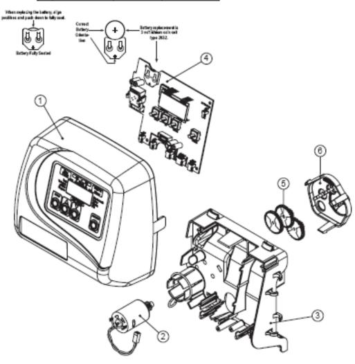
Drive Cap Assembly, Downflow Piston, Upflow Piston, Regenerant Piston and Spacer Stack Assembly
